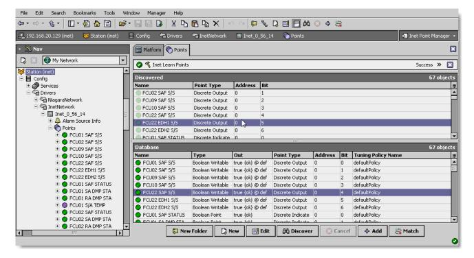
Single or multiple points can be added as control points with InetProxyExt extensions by selecting the discovered row(s) in the top pane, and clicking add. Doing so will cause the "Add" dialog box to appear: Once the point(s) are satisfactorily edited, click "OK" to create the proxy points corresponding to the point property.
