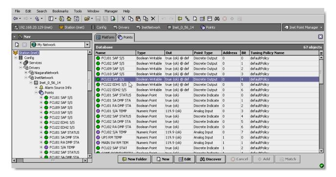
The "New Folder", "New", and "Edit" buttons are not unique to the Inet Device Manager, and are explained in the "Niagara AX User's Guide" in the "Driver Architecture" section. The "Match" button is not used for the Inet driver.
