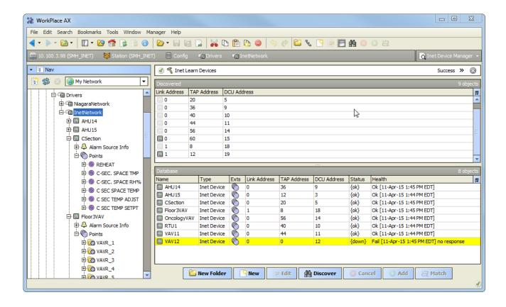
Single or multiple Inet devices can be added as device by selecting the discovered row(s) in the top pane, and clicking add. Doing so will cause the "Add" dialog box to appear:
